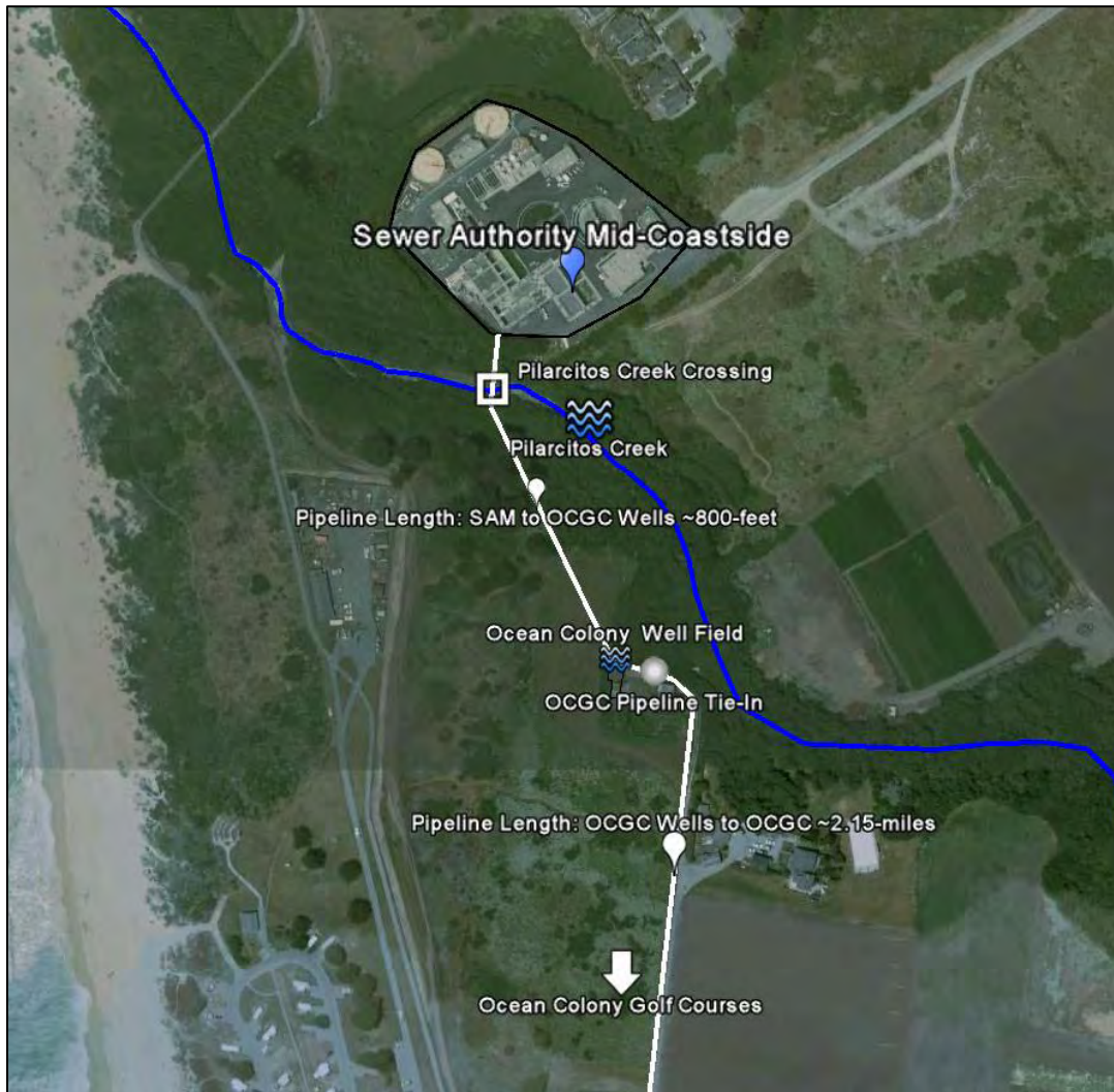
Figure 3.2 Phased Facility Pipeline
